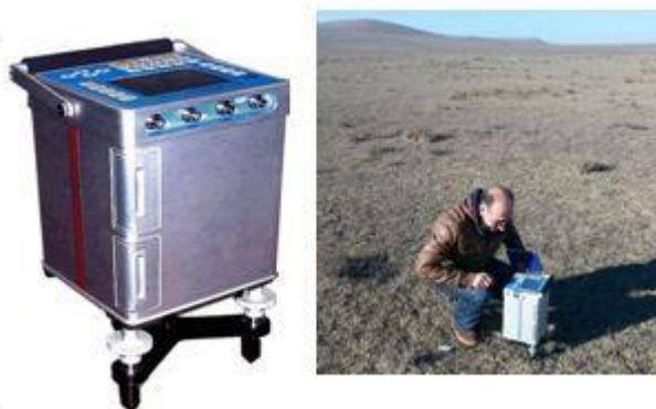
Figure 1. The view of the CG-5 AutoGrav gravimetry produced by Canada which the research works carrying out
