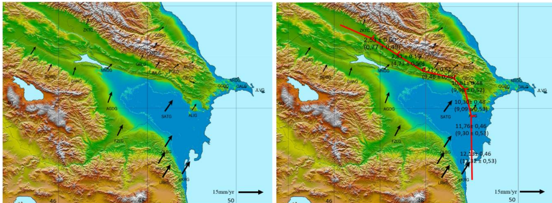
Figure 3. Horizontal velocity vector map for 2014-2022 and fault velocities (mm/yr) obtained from the block model.
