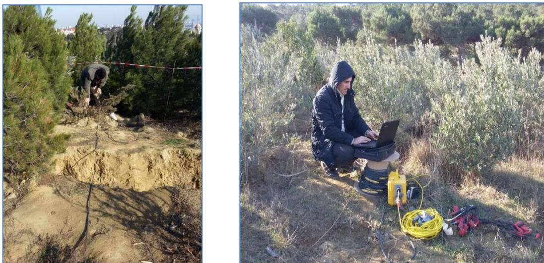
*Figure 8. Placement of seismic receivers on the profiles of the study area and registration of seismic waves*
