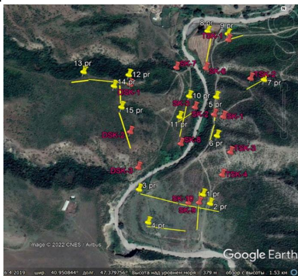
Figure 4. Location scheme of 15 seismic profiles in the research area.
