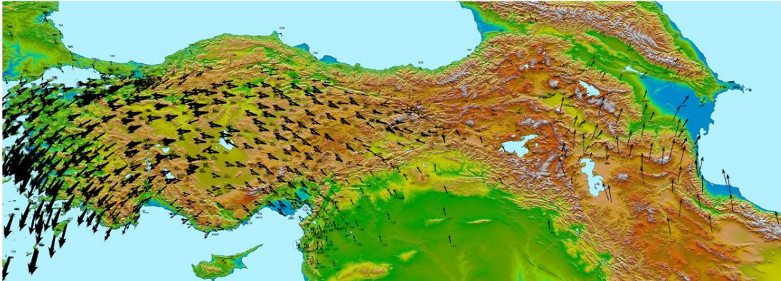
Figure 2. Map of the distribution of horizontal velocity according to the calculated GPS vectors on the territory of the Anatolian Plate and in the Caucasus for 2019-2022
