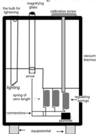
Figure 3. Scheme of gravimeter Scintrex CG-5 AutoGrav.
