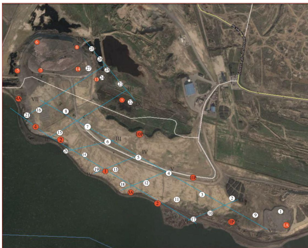
1. Scheme of location of geophysical profiles 1 Vertical Electrical Sounding points and their numbers; 2-engineering - geological boreholes and their numbers.
