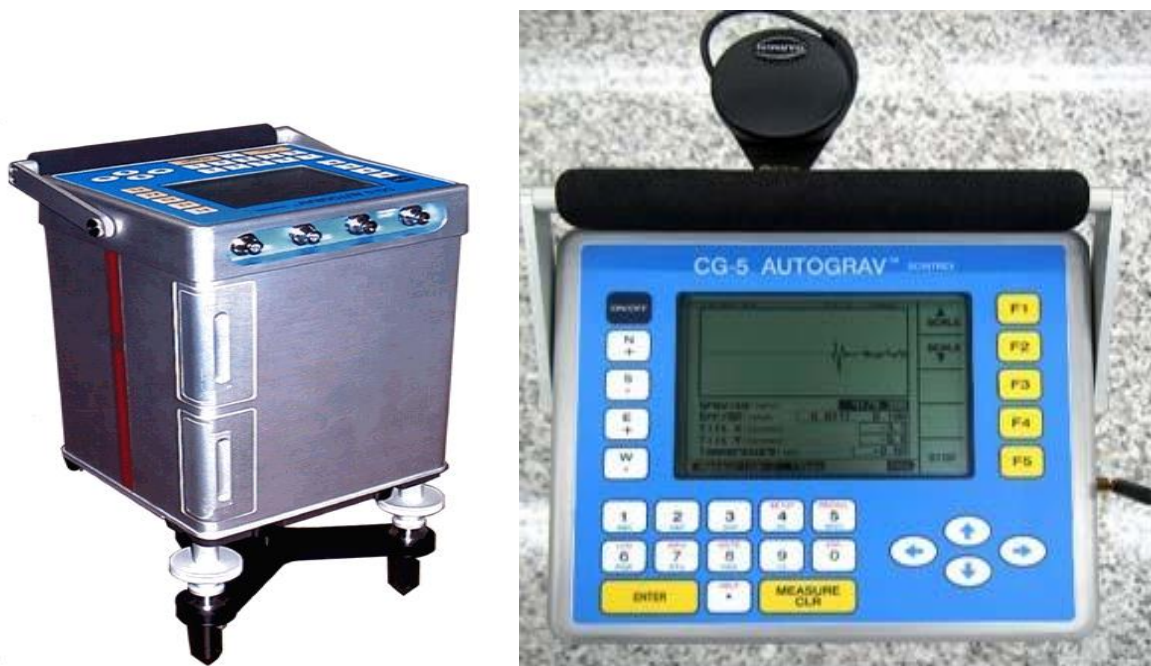
Figure 2. View of the Canadian-made CG-5 AutoGrav gravimeter under investigation.
