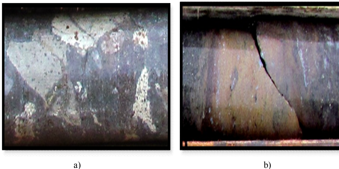
Fig. 4. a) veinlet-porous ore fold; b) vein type morphology of ore in hydrothermal changed subvolcanic rocks
