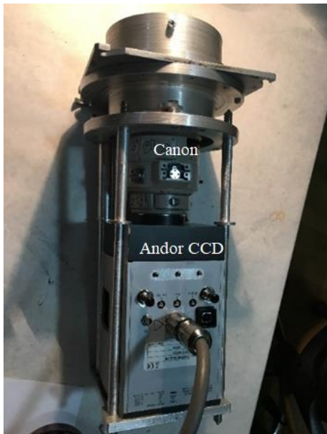
Andor CCD camera + Canon EF 200mm f / 2.0
