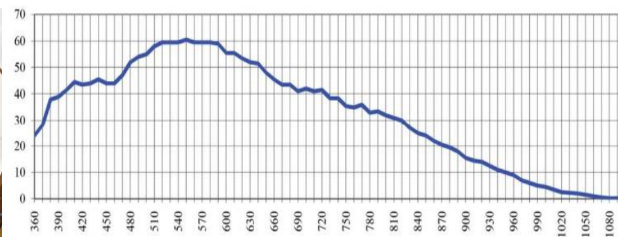
Quantum efficiency CCD FLI
