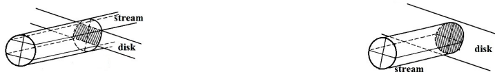
(a) The cross section of the stream is larger than vertical dimension of the disk. (b) The cross section of the stream is lower than vertical dimension of the disk
